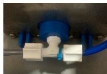
Figure 37. Rupture Disc Hose - Left of Tee at Bottom of Cell
