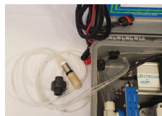
Figure 16. Brine Suction Strainer with Rupture Disc.
