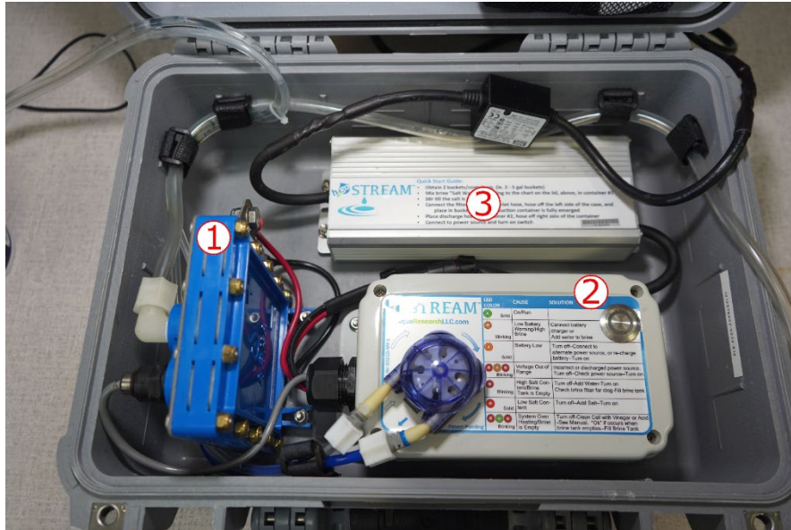
Figure 2-1. STREAM™ System Main Component Groups
