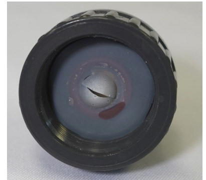
Figure 3-3. Blown Rupture Disc
