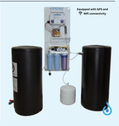
The SPRING™ Disinfectant Generator produces 1.3 lbs • (0.6 kgs) of chlorine per day, which requires 4 lbs (1.8 kgs) of salt and 3.6 kw-hrs of power.
